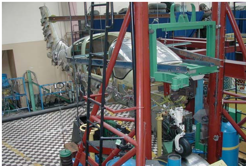
Figure 23: Airplane with nose landing gear during shimmy's tests.
