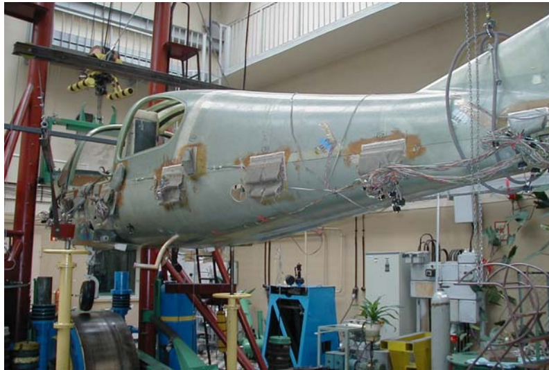
Figure 24: Airplane with nose landing gear during shimmy's tests.
